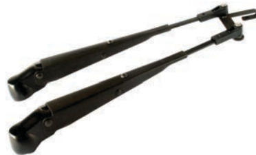
160484 Wiper Arm Mount/wiper blade 9x2.5 mm hook, Mount./wiper shaft dim. M6 cone + M8 shaft, Dist./wiper arms 57 mm, Length 340-420 mm, Length/adjustable Yes, Type Parallel Can be used together w/ wiper motor Cargo 160258, 160480.
