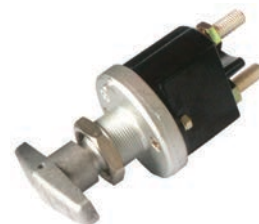
180289 Battery Main Switch 24 V, 250 A/cont., 2500 A/5 sec., Dist. mount. holes 38 mm, Type Battery, Material Metal, Protection degree IP 65, No./mount. holes 2, Key w/ Rubber boot: Cargo 180375.
