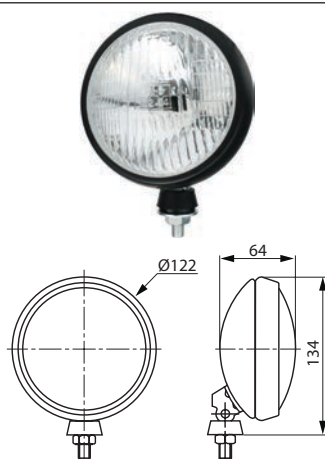
171364 Fog Lamp 12/24 V, 55/70 W, Light aperture 95 mm, Dim. 122x134x64 mm, Mount. Mounted below, Bulb type H3, Colour Black, Material Metal, Shape Round, Bulb incl. No
