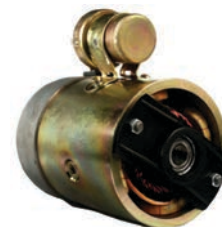
112317 DC motor 12 V, 2 kW Replacing: 11.212.622 OD 114.10, Length 191.00, Rotation CR, Not insulated return, Pulley w/o, Rpm./max. 2400
