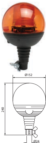
171541 Xenon Beacon 24 V, OD 152 mm, Mount. Standard ISO A - Rod, Height 240 mm, - Lens type Polycarbonat, Bulb type LX8J, Model BOULE FLASH, Colour Orange, Base Flexible, Hi impact Yes, Bulb incl. Yes, Tightness norm IP 66, E-approval Yes
