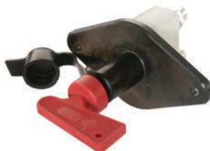
180229 Battery Main Switch 24 V, 250 A/cont., 2500 A/5 sec., Dist. mount. holes 100 mm, Type Battery, Material Plastic, Protection degree IP 66, No./mount. holes 2, Key w/
