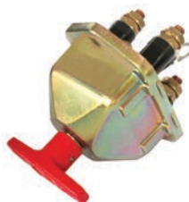
180276 Battery Main Switch 24 V, 250 A/cont., 2500 A/5 sec., Dist. mount. holes 110 mm, Type Battery, Material Plastic, Protection degree IP 67, No./mount. holes 2, Poles 2, Explosion proof 1 Yes, Explosion proof 2 Yes, Waterproof Yes, Key w/ Rubber boot: Cargo 180375. For alternator w/intergal regulator. w/D+ contact.
