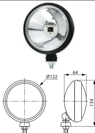
171363 Driving Lamp 12-24 V, Light aperture 95 mm, Dim. 122x134x64 mm, Mount. Mounted below, Bulb type H3, Colour Black, Material Metal, Shape Round, Bulb incl. No
