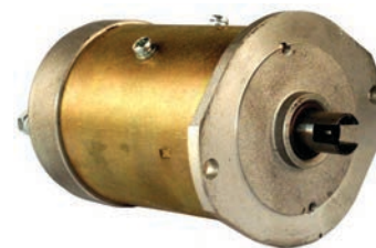
112484 DC Motor 24 V, 0.4 kW Replacing: 19024741, 19024720 OD 79.60, Length 167.50, Rotation CR, Pulley w/o, Rpm./max. 3300 Permanent magnet.
