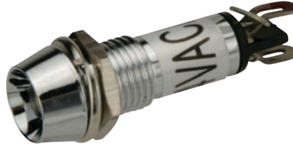
181574 Indicator Light 12/24 V, Mount. hole size 8 mm, Type/terminal Solder, Colour White, Material Nickel plated brass, Bulb LED
