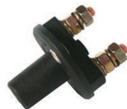
180313 Battery Main Switch 24 V, 100 A/cont., 500 A/5 sec., Dist. mount. holes 45 mm, Type Battery, Protection degree IP 4x, No./mount. holes 2, Key w/o Spare key: Cargo 180143. Rubber protection cap: Cargo 180374.
