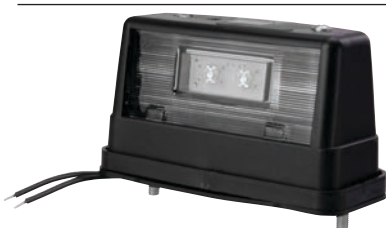
171709 LED Numberplate Lamp 12/24 V, Dim. 109x61x55.5 mm, Type LED, Socket type LED, Colour Red, Material Shockproof plastic, Fixing screw 2, Numberplate light w/ E-approval Yes
