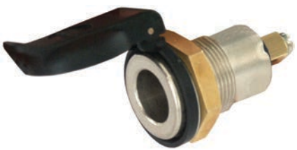
180038 DIN Socket ID/mount. hole 18.5 mm, Material Nickel plated brass, Connection Screw, No./mount. holes 1, Bracket w/ Female, DIN norm 72591, ISO norm 4165 Standard DIN.
