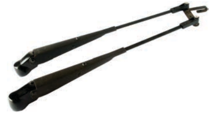
160485 Wiper Arm Mount./wiper blade 9x2.5 mm hook, Mount./wiper shaft dim. M8 cone + M8 shaft, Dist./wiper arms 57 mm, Length 430-500 mm, Length/adjustable Yes, Type Parallel
