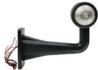
171530 LED Tail-Position Lamp 24 V, Dim. 115x65x48 mm, Dist. mount. holes 73 mm, Mount. 2 screws, Cable length 700 mm, Type LED, Colour/glass Red/white, Material Rubber, Material/dome Shockproof plastic, Fixing screw 6, Connection Cable, LEDs w/, LEDs 2 2x1, Sidemarker w/, Tail light w/, RH/ LH RH/LH, E-approval Yes
