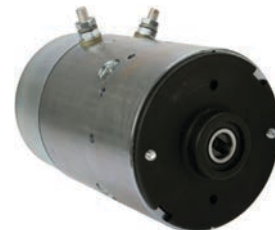
112311 DC Motor 12 V, 2.1 kW Replacing: amj5667, 11.212.108 OD 112.25, Length 196.75, Rotation ACR, Insulated return, Pulley w/o, Rpm./max. 1700
