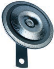
160393 Horn 36-48 V, 335 Hz, OD 100 mm, Type Single tone, E-approval Yes 2 terminals. w/ bracket.
