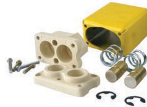
180577 Battery Connector 250 V, 300 A, Cable dim. 70 mm 2 , Mount. Soldering, Model E300, Colour Yellow, Material 2 Copper alloy, Bracket w/ Shells: stamped steel and coated w/yellow paint. Insulators: DMC mouldings. Terminals w/brazed solid silver tip.
