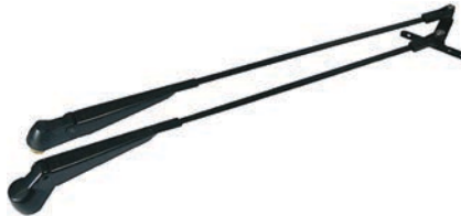
160358 Wiper Arm Mount./wiper shaft dim. M6 cone + M8 shaft, Dist./wiper arms 57 mm, Length 500 mm, Length/adjustable No Usable w/wiper motor: Cargo 160258, 160290, 160291, 160357, 160408.
