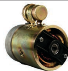
112317 DC motor 12 V, 2 kW Replacing: 19024743, 19024730 OD 114.10, Length 191.00, Rotation CR, Not insulated return, Pulley w/o, Rpm./max. 2400
