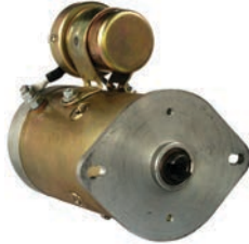
112522 DC Motor 12 V, 0.8 kW Replacing: 19024663 OD 78.50, Length 175.00, Rotation CR, Rpm./max. 2700
