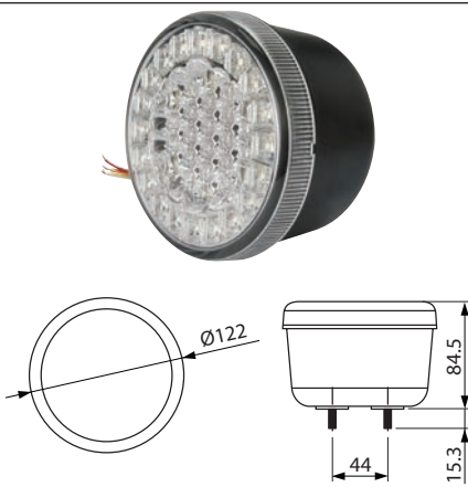
171726 LED Fog/Reverse Lamp 12/24 V, Dim. 122x84.5 mm, OD 122 mm, Dist. mount. holes 44 mm, Cable length 150 mm, Type LED, Material Shockproof plastic, Material/ dome Shockproof plastic, Connection Cable, LEDs w/, LEDs 2 38, Numberplate light w/o, Rear/fog lamp w/, Reverse light w/, Reflector w/o, E-approval Yes Ring: clear, center: red.
