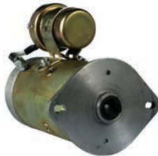
112523 DC Motor 24 V, 1.2 kW Replacing: 19024668 OD 79.50, Length 175.50, Rotation CR, Pulley w/o, Rpm./max. 3200
