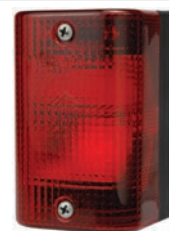
170930 Rear Fog Lamp 21 W, Dim. 125x84x68 mm, Socket type BA15S, Colour Black, Material Shockproof plastic, Fixing screw 1, Connection Connection, Rear/fog lamp w/, Bracket Pendant, E-approval Yes
