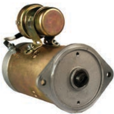
112520 DC Motor 12 V, 0.8 kW Replacing: 19024676 OD 78.50, Length 175.00, Rotation CR, Rpm./max. 2700
