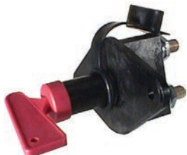
180203 Battery Main Switch 24 V, 250 A/cont., 2500 A/5 sec., Dist. mount. holes 100 mm, Type Battery, Material Plastic, Protection degree IP 66, No./mount. holes 2, Key w/
