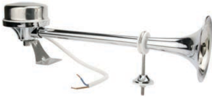
160414 Horn 24 V, 118 dB, 370 Hz, Length 455 mm, Type Single tone, Material Chromed Brass, Marine Yes Model em2.
