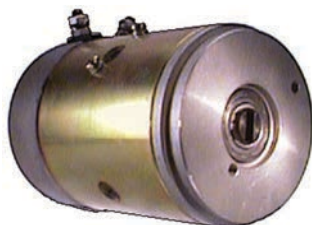
111092 DC Motor 12 V, 2 kW Replacing: 0136355080 OD 117.30, Length 195.45, Rotation CR, Insulated return, Pulley w/o, Rpm./max. 2400
