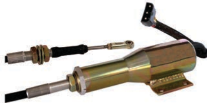
090267 Shutdown Solenoid Servicing: Volvo wheel loader 24 V, 0.86 A/hold, 39 A/pull, Pull rating 129N at 25.4mm, Hold rating 182N, Elect. connection Multiplug, Function Pull, Plunger Cable Syncro start / Woodward.
