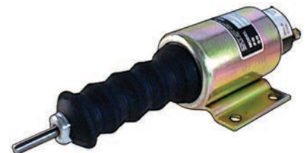
090169 Shutdown Solenoid Servicing: Universal. 24 V, 0.3 A/hold, 23 A/pull, Thread size 6, Thread type mm, Pull rating 75N at 25.4mm, Hold rating 178N, Elect. connection Connection, Function Pull, Plunger External, Switch Internal, Return spring 35N Syncro start / Woodward.
