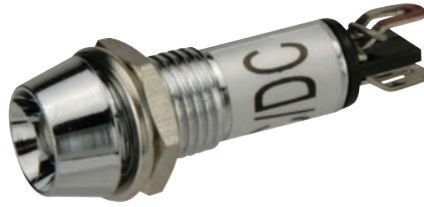
181573 Indicator Light 12/24 V, Mount. hole size 8 mm, Type/terminal Solder, Colour Blue, Material Nickel plated brass, Bulb LED
