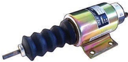
090113 Shutdown Solenoid 24 V, 0.3 A/hold, 23 A/pull, Th read size 6, Thread type mm, Pull rating 75N at 25.4mm, Hold rating 178N, Elect. connection Connection, Function Pull, Plunger External, Return spring 35N Syncro start / Woodward.
