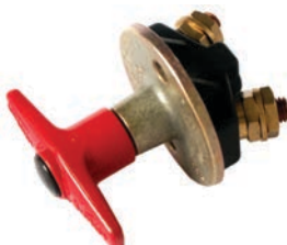
180271 Battery Main Switch 12/24 V, 300 A/cont., 1000 A/5 sec., Dist. mount. holes 45 mm, Type Battery, Material Plastic, Protection degree IP 65, No./mount. holes 2, Poles 10, Explosion proof 1 Yes, Waterproof Yes, Key w/, Approval SAE J1171 Rubber boot: Cargo 180375. Working temp. -30°C / +65°C.
