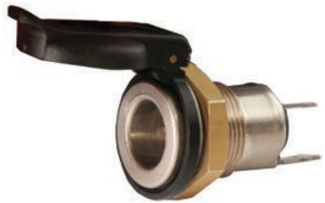
180157 DIN Socket ID/mount. hole 18.5 mm, Material Nickel plated brass, Connection Terminal, No./poles 2, Bracket w/, Female, DIN norm 72591, ISO norm 4165
