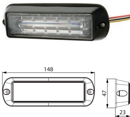
171662 LED Flash, amber 12/24 V, Length 148 mm, Height 23 mm, Width 47 mm, Lens type Clear, Bulb type LED, Model 6 LED, Colour Orange, Waterproof Yes, Approvals SAE/CE, E-approval Yes 19 flash patterns. Multi-module synchronization. Bracket: Cargo 171664.
