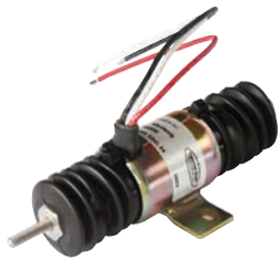
090200 Shutdown Solenoid 24 V, 4 A/hold, 18 A/pull, Th read size 6, Thread type mm, Pull rating 67N at 25.4mm, Hold rating 178N, Elect. connection Cable, Function Pull/push, Plunger External, Return spring 17N Syncro start / Woodward. Red=hold. White=pull. Black=ground.
