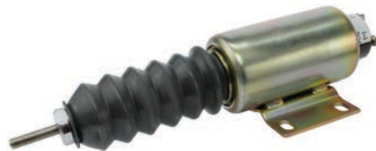
090431 Shutdown Solenoid Servicing: Universal. 24 V, 24 V 2, 0.57 A/hold, 30 A/pull, Thread size 5/16 \times - 24, Thread type Inches, Pull rating 165N, Hold rating 391N, Function Pull, Plunger External, Insulated return, Return spring 17.6 - 26 lbs Syncro start / Woodward.
