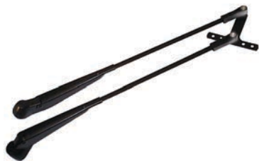
160257 Wiper Arm Mount./wiper shaft dim. M6 cone + M8 shaft, Dist./wiper arms 57 mm, Length 400 mm, Length/adjustable No, Type Parallel Usable w/wiper motor: Cargo 160258, 160290, 160291, 160357, 160408.
