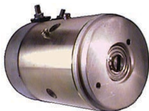
111091 DC Motor 24 V, 2.5 kW Replacing: 0136355081 OD 117.00, Length 195.60, Rotation CR, Insulated return, Pulley w/o, Rpm./max. 2100
