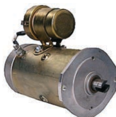
112138 DC Motor 12 V, 0.8 kW Replacing: ame1706, ame1609, 11.212.192, 11.212.147 OD 78.00, Length 184.00, Rotation CR, Not insulated return, Pulley w/o, Rpm./max. 2700
