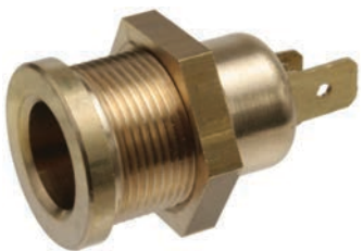
180377 DIN Socket Servicing: Cargo 170292, 170387, 170405, 170788, 170406, 170562, 170789, 170537, 171576, 170419 170460. Mount. hole size 18 mm, Socket DIN 72591 2 terminal 2-pole flat plug.
