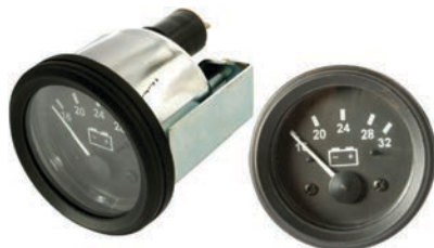
160696 Voltmeter 16-32 V, OD 52 mm, Measuring unit v, Measuring range 16-32, Mount. type Hook fastening, Colour Black White figures.
