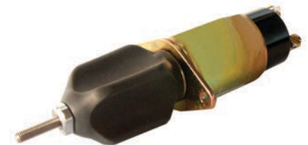
090297 Shutdown Solenoid 24 V, 1.1 A/hold, 46 A/pull, Thread size 6, Thread type mm, - Pull rating 107N at 25.4mm, Hold rating 169N, Plunger External, Return spring 7-11N
