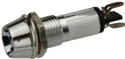
181572 Indicator Light 12/24 V, Mount. hole size 8 mm, Type/terminal Solder, Colour Yellow, Material Nickel plated brass, Bulb LED
