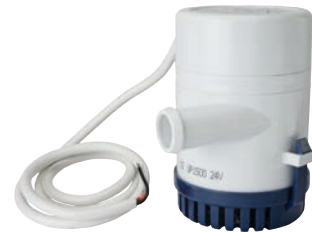
070185 Bilge Pump 24 V, Dim. 160x96 mm, Hose connection 26.5, Lift height 4 m, Type Bilge, Pump housing ABS plastic, Pump shaft Stainless steel, Capacity 95 l/min, Gasket Ceramic Model UP1500. Completely submersible bilge pump. Compact design w/ABS material housing, corrosion resistant. Shaft seal made of ceramic and graphite which ensures lubrication and leak resistance. Water inlet strainer slots will screen particles present in the bilge allowing easy running. Pump body can be dismantled by a simple snap - off movement for easy inspection and cleaning.
