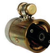
112318 DC Motor 24 V, 2.5 kW Replacing: 11.212.619 OD 114.14, Length 191.25, Rotation CR, Not insulated return, Pulley w/o, Rpm./max. 2100
