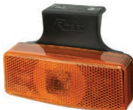
170884 Side Marker Lamp 5 W, Dim. 110x46x26 mm, Dist. mount. holes 85 mm, Socket type T10, Colour/glass Orange, Material Shockproof plastic, Fixing screw 2, Shape Rectangular, Connection Connection, Reflector w/ , E-approval Yes Lens: Cargo 170946.
