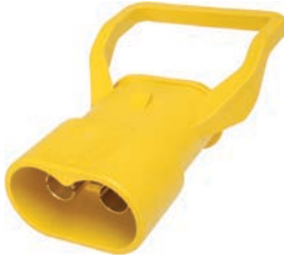
180580 Battery Connector 150 V, 250 A, Cable dim. 50 mm 2 , Mount. Soldering, Type Male, Model Y250, Colour Yellow, Material Thermoplastic, Material 2 Copper alloy
