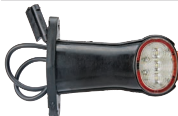
171617 LED Tail-Position Lamp 9-36 V, Dim. 96x76x63 mm, OD 76 mm, Dist. mount. holes 78 mm, Type LED, Colour/glass Red/white, Material Synthetic rubber, Connection Cable, LEDs w/, LEDs 2 2x3, Sidemarker w/, Tail light w/, Reflector w/o, RH/ LH RH/LH, Approvals ADR/SAE, E-approval Yes
