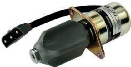
090226 Shutdown Solenoid 24 V, 24 V 2, 0.5 A/hold, 25 A/pull, Thread size 6, Thread type mm, Pull rating 111N at 25.4mm, Hold rating 182N, Elect. connection Multiplug, Function Pull, Plunger Internal, Return spring 7N Syncro start / Woodward. Red=Common. White=Pull. Yellow=Hold.
