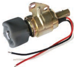
090371 Shutdown Solenoid Servicing: Kubota D722, Z482 24 V, 0.5 A/hold, 25 A/pull, Elect. connection Cable
