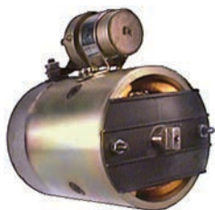
110429 DC Motor 12 V, 2 kW Replacing: amj5632, 11.212.066 OD 115.00, Length 174.00, Rotation CR, Not insulated return, Pulley w/o, Rpm./max. 2400
