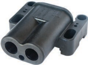
180581 Battery Connector 250 V, 250 A, Cable dim. 50 mm 2 , Mount. Soldering, Type Female, Model P250, Colour Black, Material Thermoplastic, Material 2 Copper alloy
