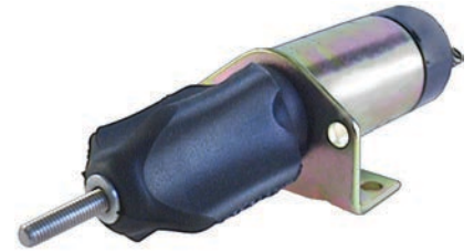
090161 Shutdown Solenoid Servicing: Universal. 24 V, 0.25 A/hold, 17 A/pull, Thread size 6, Thread type mm, Pull rating 40N at 25.4mm, Hold rating 89N, Elect. connection Connection, Function Pull, Plunger External, Return spring 17N Syncro start / Woodward.
