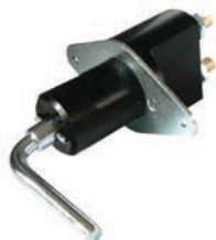
180087 Battery Main Switch 24 V, 250 A/cont., 2500 A/5 sec., Dist. mount. holes 100 mm, Type Battery, Material Metal, No./mount. holes 2, Key w/ Spare key: Cargo 180202.
