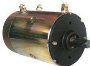
112575 DC motor 24 V, 2 kW Replacing: 0136501074 OD 112.25, Length 226.50, Rotation CR/ACR, Not insulated return, Pulley w/o, Rpm./max. 2400
