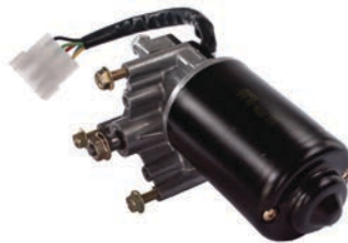
160408 Wiper Motor 24 V, Wiper angel 95°, Dist./shafts 57 mm, Wiper shaft w/2 shafts for parallelogram, Type Universal, Auto stop Yes w/ reciprocating shaft.
