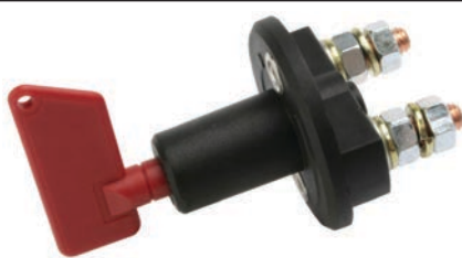
180216 Battery Main Switch 24 V, 100 A/cont., 500 A/5 sec., Dist. mount. holes 45 mm, Type Battery, Material Plastic, Protection degree IP 4x, No./mount. holes 2, Key w/ Spare key: Cargo 180143. Rubber protection cap: Cargo 180374.
