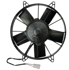
160906 Axial Fan 24 V, Dia. 225 mm, Type Suction, Capacity 1060 m 3
