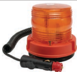
171541 Xenon Beacon 24 V, OD 152 mm, Mount. Standard ISO A - Rod, Height 240 mm, - Lens type Polycarbonat, Bulb type LX8J, Model BOULE FLASH, Colour Orange, Base Flexible, Hi impact Yes, Bulb incl. Yes, Tightness norm IP 66, E-approval Yes
