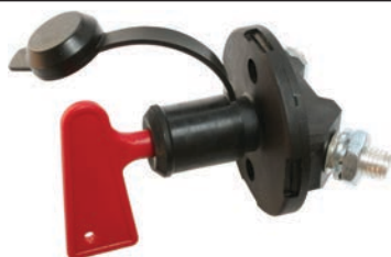
180028 Battery Main Switch 24 V 2, 100 A/cont., 500 A/5 sec., Dist. mount. holes 38 mm, Type Battery, Material Plastic, No./mount. holes 2, Key w/ Spare key: Cargo 180143. Pole: \varnothing 10 mm.
