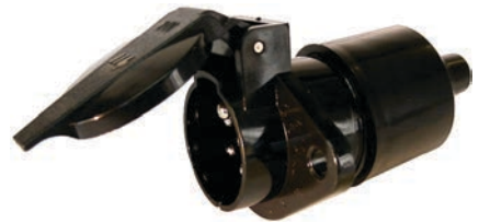
180112 Trailer Socket Servicing: Cargo 180296, 180351, 180111, 180154 24 V, Plug type 24N, Europe, Colour Black, Material Shock thermo plastic, Connection Terminal, No./poles 7, Female, DIN norm 72579, ISO norm 1185
