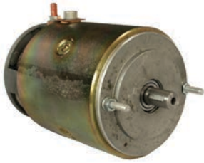
112508 DC Motor 12 V, 1.8 kW Replacing: 19024650 OD 114.50, Length 198.30, Rotation CR, Pulley w/o, Rpm./max. 2600
