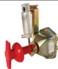
180279 Battery Main Switch 24 V, 250 A/cont., 2500 A/5 sec., Dist. mount. holes 110 mm, Type Battery, Material Plastic, Protection degree IP 65, No./mount. holes 2, Poles 1, Pneumatic Yes, Explosion proof 2 Yes, Key w/ Rubber boot: Cargo 180375. Spare key: Cargo 180292.
