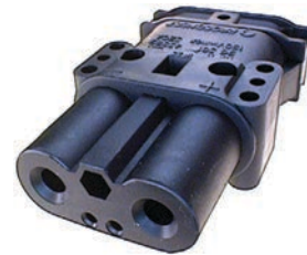
180395 Battery Connector 150 V, 320 A, Cable dim. 90 / 70 mm 2 , Mount. Solder/crimp, Type Female, Model NF320, Colour Black, Material Plastic, Material 2 Silver plated copper alloy, Temp./max + 90°C, Temp./min - 20°C, Protection degree IP 23, Resistant to acid Yes w/reducing bushings for 70 mm 2 cable.
