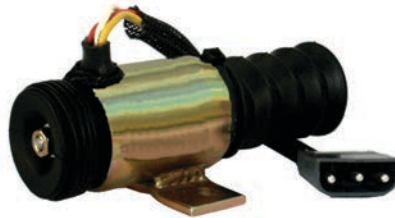
090281 Shutdown Solenoid Servicing: Volvo 24 V, 0.5 A/hold, 25 A/pull, Thread size 6, Thread type mm, Pull rating 89N at 25.4mm, Hold rating 236N, Elect. connection Multiplug, Function Pull/push, Plunger Internal Syncro start / Woodward.
