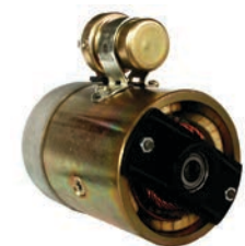
112318 DC Motor 24 V, 2.5 kW Replacing: 19024732, 19024731 OD 114.14, Length 191.25, Rotation CR, Not insulated return, Pulley w/o, Rpm./max. 2100
