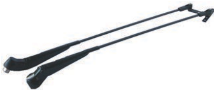
160256 Wiper Arm Mount./wiper shaft dim. M6 cone + M8 shaft, Dist./wiper arms 57 mm, Length 450 mm, Length/adjustable No Usable w/wiper motor: Cargo 160258, 160290, 160291, 160357, 160408.
