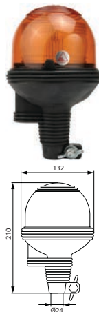
171614 Xenon Beacon 10-30 V, OD 132 mm, Mount. Standard ISO A - Rod, Height 210 mm, Lens type Polycarbonat, Bulb type LX10J, Model Xenon, Colour Orange, Hi impact Yes, Bulb incl. Yes, E-approval Yes
