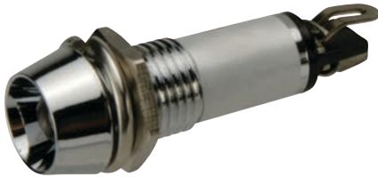
181570 Indicator Light 12/24 V, Mount. hole size 8 mm, Type/terminal Solder, Colour Red, Material Nickel plated brass, Bulb LED En60947-5-1, IEC947-5-1.
