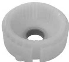
139323 Outer Gear Replacing: m135x01571, m135x01471 Servicing: M000T60081, M000T60081A, M000T60181, M000T60181A, M000T65381, M000T80081, M000T80281, M000T80281A, M000T80281B ID 46.90, OD 63.80, No./ teeth 42 Bushing I.D. 17.50 mm.
