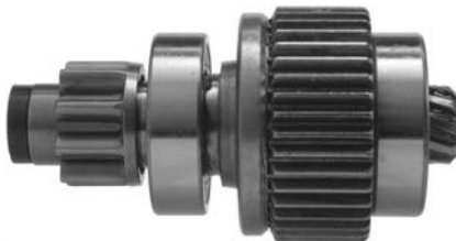
238986 Drive Servicing: 03101-3050 OD 29.20, Total length 104.00, Splines A 10, No./ teeth 9
