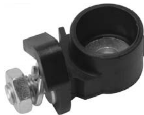
236782 B+ terminal Servicing: M000T87681, M000T90981, MOT87681, m0t90981 Total length 46.00, Thread length 13.40, Thread size M8
