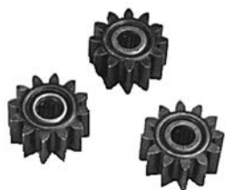
139572 Gear Wheel Kit ID 5.00, OD 18.00, Height 9.50, No./ teeth 12 Alternative no.: b139572
