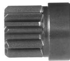
134237 Dp Gear ID 12.00, OD 25.10, Height 32.35, No./ teeth 9
