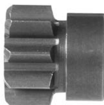
134169 Dp Gear ID 12.10, OD 25.20, Height 24.90, No./ teeth 9
