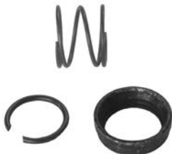
235003 Stop Collar Kit Servicing: M008T61671, M8T61671 ID 15.10, OD 19.40/20.80, Height 5.90
