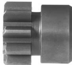
134190 Dp Gear ID 14.00, OD 34.60, Height 36.90, No./ teeth 9
