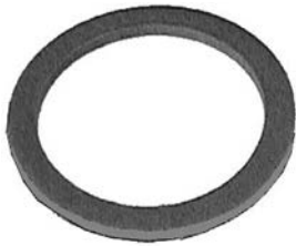
134764 Fiber Washer Replacing: 1000207006 Servicing: 00010DB98E, 0001106011, 0001106012, 0001106014, 0001106015, 0001106016, 0001106017, 0001106018, 0001106019, 0001106022 ID 18.50, OD 23.50, Thickness 1.60, Material Fiber
