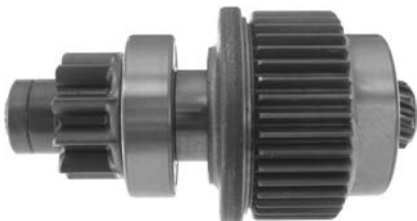
235095 Drive Servicing: 03111-4140, 03111-4240, 03111-4241 OD 32.00, OD/ housing 42.00, Total length 104.00, Splines A 10, No./ teeth 10
