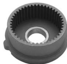
235502# Outer Gear Replacing: me701486, m135x07711 Servicing: M008T50071, M008T50171, M008T80071, M008T80071A, m8t50071, m8t50171, m8t80071, m8t80071a, m8t80171, m8t85071, m8t85071a OD 61.80/69.80, Height 30.90, No./ teeth 44 w/ bushing. Needle bearing: HC-CARGO 141065.
