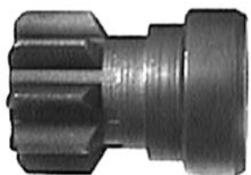
137012# Gear Wheel ID 12.00, OD 25.45, Height 36.40, No./ teeth 9
