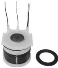
138934 Solenoid Coil 12 V, ID 21.00, OD 46.55
