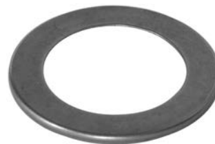
134229# DP Washer ID 25.75, OD 38.50, Thickness 1.60, Material Steel
