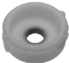
139199 Outer Gear Replacing: md618538, m135x00871 Servicing: M000T70281, M000T70285, M000T70381, M000T71385, M000T71581, M000T71681, M000T71786, M000T71881, M000T86681, M0T70281 ID 48.95, OD 64.00, Height 30.60, No./ teeth 43
