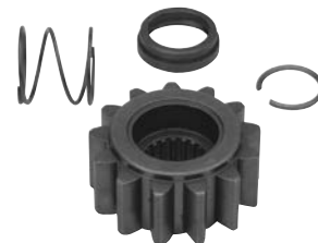
237086 Pinion Servicing: HQ808670, MG122202, mg122433, TM000A18601 ID 13.74, OD 39.51, Height 18.27, Splines 19, No./ teeth 13
