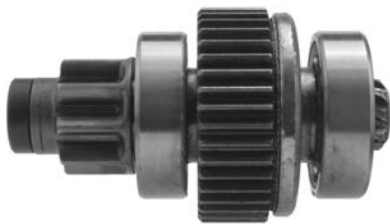
236607 Drive Servicing: 03101-3170, 03101-3190, 03101-3220 OD 29.00, Total length 93.50, Splines A 10, No./ teeth 9, Rotation CR
