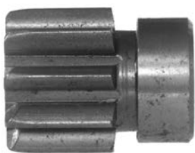
134233 Dp Gear ID 12.10, OD 25.00, Height 32.60, No./ teeth 9
