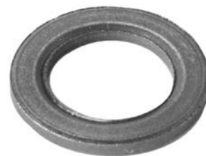
134223 DP Washer Replacing: 1000103005 Servicing: 1006209570 ID 12.35, OD 19.65, Thickness 2.00, Material Steel
