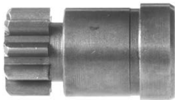
134172 Dp Gear ID 12.00, OD 25.60, Height 48.25, No./ teeth 9
