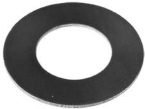
134758 DP Washer ID 29.25, OD 53.85, Thickness 1.60, Material Fiber
