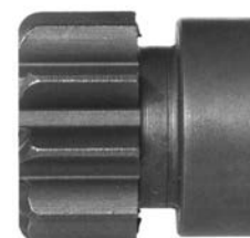
134185 # Dp Gear ID 12.00, OD 27.70, Height 28.65, No./ teeth 10
