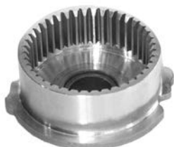
233638 Outer Gear Servicing: M000T80082, M001T80081, M001T80082, m0t80082, m1t80081, m1t80082 ID 46.30, OD 55.80, Height 30.32, No./ teeth 42 Bearing: HC-CARGO 140920.
